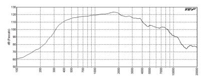
Low Frequency Protection: The LH-30TA is not designed to operate below 300 Hz. Head-end processing equipment should include a 300 Hz high-pass filter with a roll-off of 6dB per octave to limit the low frequency input to the horn. If head-end processing is not available, an alternate method of providing low frequency protection for the horn driver is to insert one non-polarized series capacitor at the high side input [terminal 2 (+)] of each horn.
