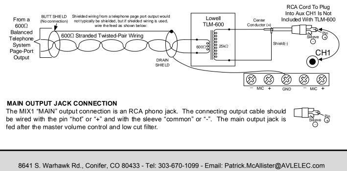
The MIX1 balanced "MIC" level and "LINE" level outputs are available at screw terminals. These outputs are fed after the master volume control and low cut filter.
